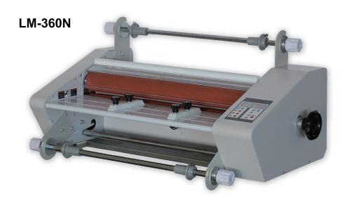
Tabletop hot and cold roll laminating machine, designed for professional usage.
